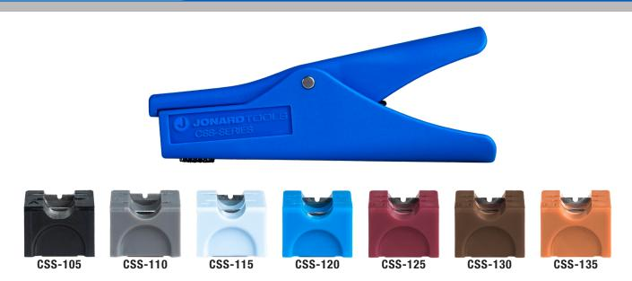
The CSS Series tools are coaxial cable strippers specifically designed to strip a stub end of a coax cable in a wall outlet box, which eliminates the need to run new cable, saving time and money. Each strips RG-59 and RG-6 cables to specific braid and center conductor lengths shown in chart below. The built-in strip stop insures the strip lengths are consistent. VELCRO® strip on bottom of tool is used to fold back braid on cable after being stripped.
