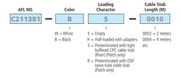
Example: Order number for a panel Black in color, loaded with 72 PSC adapters (12 six packs), connectors and a cable stub 10 meters in length.
