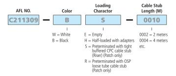
**Example:** Order number for a panel Black in color, loaded with 48 PSC adapters (8 six packs), connectors and a cable stub 10 meters in length.
