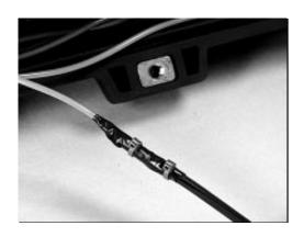
6.10 Install the FibrTube in the organizer tray by pressing the tube in the channel with the two ridges facing up. The end of the FibrTube should not extend into the fiber routing area of the tray.
