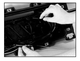
6.3 Orient the FibrTube with the two ridges facing up.
