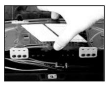
9.3 Remove the backing from the hook tabs. Attach the tabs to the sides of the trays.
