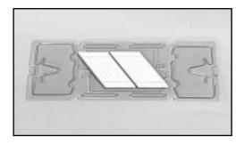
5.2.3 Install the splice tray in the closure. The tray has two holes which accommodate #8-32 screws, and a flat surface on the bottom for adhesive type fasteners. The method for fastening the tray is usually supplied with the closure.
