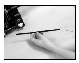
6.9 Place the 3M<sup>™</sup> FibrTube over the buffer tube with a 1 in. (2.5 cm) overlap. Use a cable tie and/or vinyl tape to secure the FibrTube to the buffer tube.
