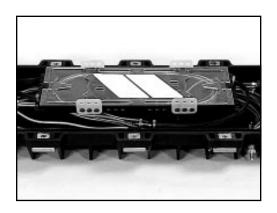
8.2 Position another tray on top of the first one. Make sure each set of knobs lines up with the ones below. The trays should be nested.
