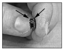
6.4 Allow for a 1 in. (2.5 cm) overlap between the FibrTube and the buffer tube.
