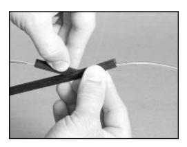
6.8 Ensure the FibrTube runs freely over the fibers. If necessary, unzip the tubing and repeat the process in step 6.7. Remove the installation tool.
