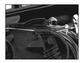
6.11 Secure the FibrTube with a cable tie.
