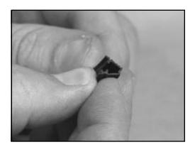
6.7 Install the fibers into the FibrTube.
